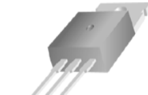
TO-220 Pin Definition 1. Base 2. Collector 3. Emitter
